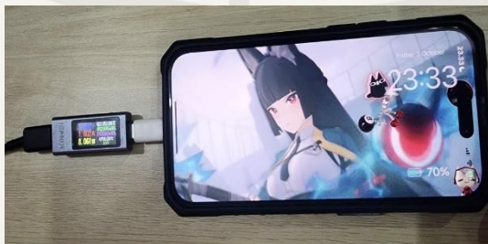
Figure 3. Charging Process of 70% SoC (With the Charger, USB Power Meter Dongle, and Lightning Connector connected to the device)
