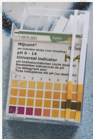
Figure 4. Results of pH testing using Universal Indicator on filtered lake water samples (Source: private)
